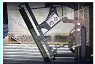
“Locks” the load to the pallet by rolling film into a tight cable and driving it down onto the bottom of the load.
