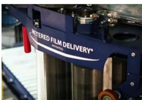
Doubles the wrap force per revolution without crushing or twisting the load; also reduces film breaks.
