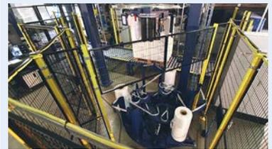
ARC limits roll changes, works with all films regardless of variable film fluctuations and minimizes clogging of the film delivery system, all of which limits the need for operator touches.
