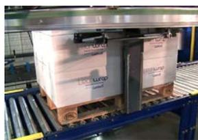
Load-Seeking Clamp guards against film pull-outs and tear-outs; also reduces film breaks and seals the film tail to the load.
