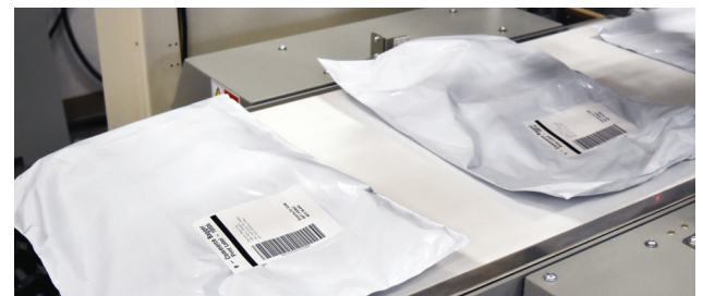
LABELS WITH BAR CODES & ADDRESS AUTOMATICALLY APPLIED
